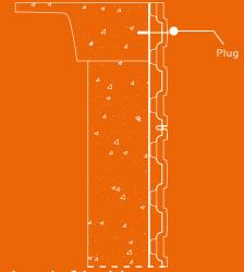
Fasten the top panel with a plug (prefer chemical over mechanical ones) near the curb of the slab.
