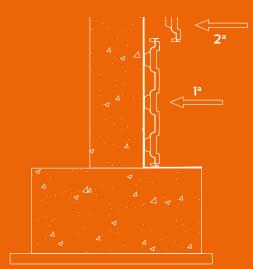
After installation of the waterproofing, begin the installation of DEFENDER as in the image on the right.
