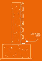
$Lay\ a\ drainage\ pipe\ along\ the\ perimeter\ of\ the\ building\ and\ close\ to\ the\ wall\ to\ discharge\ water\ into\ a\ drainage\ basin.$
