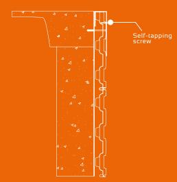
$Place \ the \ corrugated \ plastic board \ sheet \ on \ top \ of \ DEFENDER \ panels \ and \ fasten \ them \ with \ self-tapping \ screws.$
