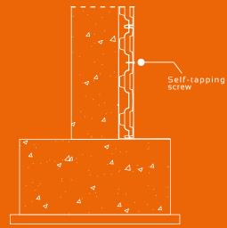
Apply a sheet of plasticboard near the corners and fasten it to DEFENDER with self-tapping screws (50 mm or less). www.geoplast.it
